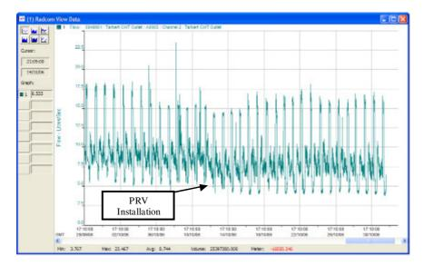
As you can see a nightline reduction of 1.2 l/sec has been attained through pressure control.
